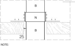
The optional support brace (N) has the ability to adjust to any angle of adjacent roof beams
