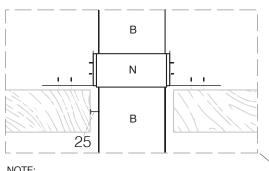
The optional support brace (N) has the ability to adjust to any angle of adjacent roof beams
