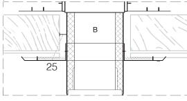
\*There is a 25mm clearance between the flue and any timber at all times\*
