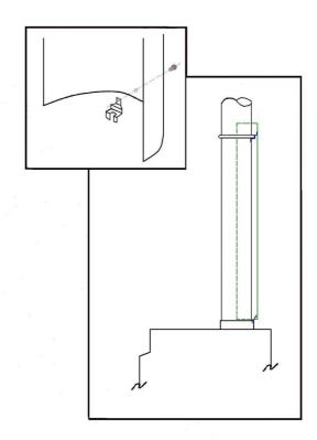
Fit the next length of flue pipe, trapping the top bracket and complete the flue installation as described in the instructions supplied in the kit.
